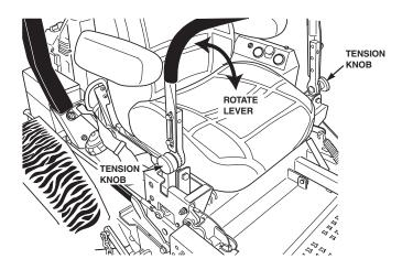
Figure 4-7. Adjusting Steering Levers
